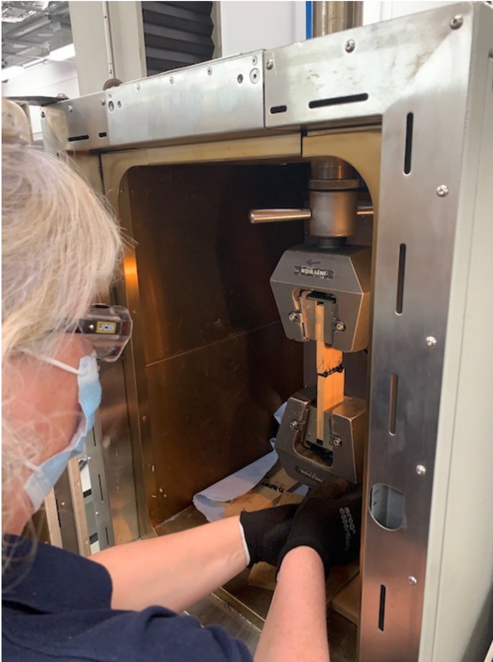
Samantha Hambrook sets up 70 degree tensile pull test on a caulking sample. Courtesy of the University of Southampton.
